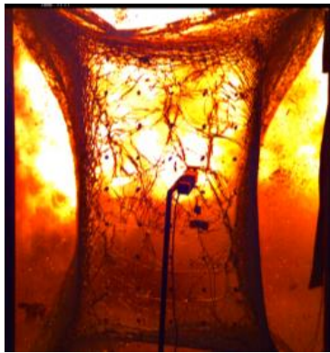
c) Boundary failure [93]
