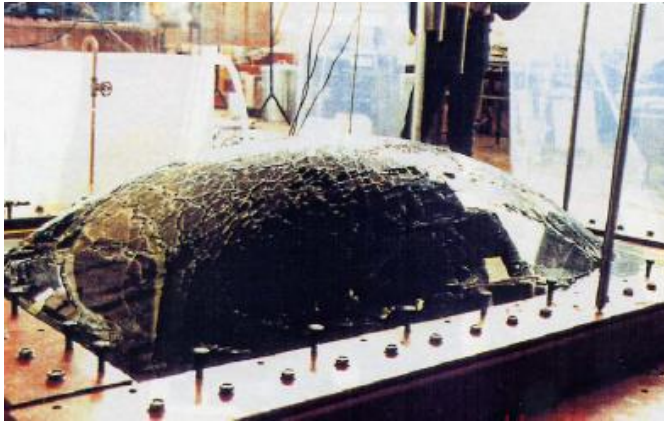
a) Quasi-static waterbag test [92]
