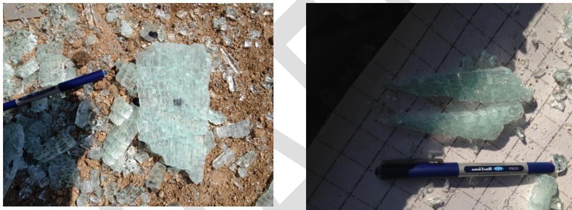
b) Large pieces of squared and slender fragments from tempered glass windows [71]
