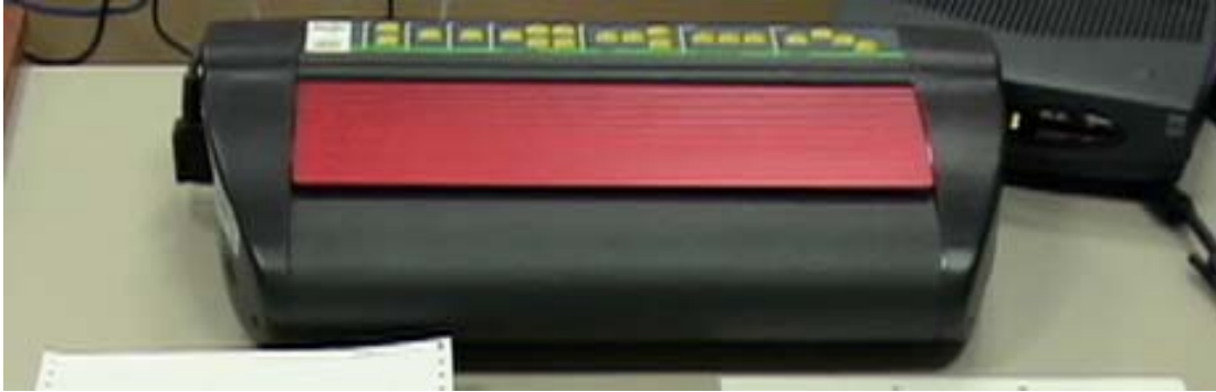
Figure 5.1: Index Basic D Braille embosser.
