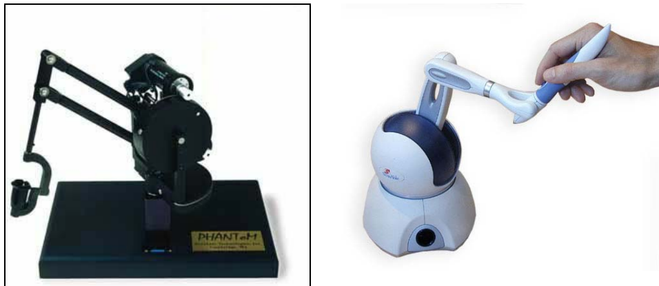
Figure 2.6: The PHANToM (left), the PHANToM Omni (right) Source :
