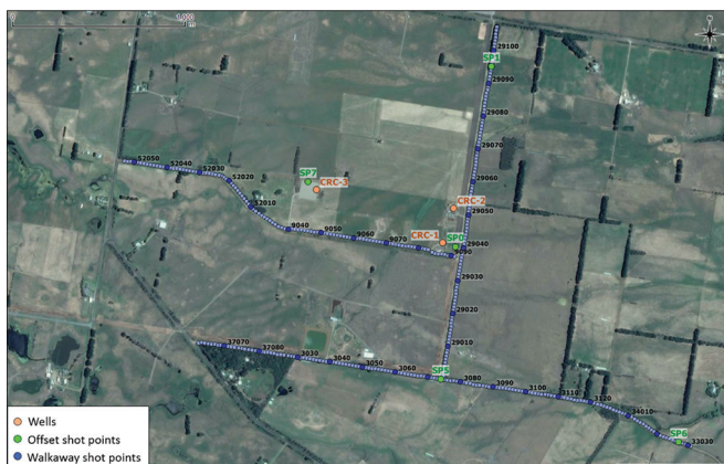
Figure 1. Survey map for the VSP acquisition in CRC-3 well, C02CRC Otway research site.
