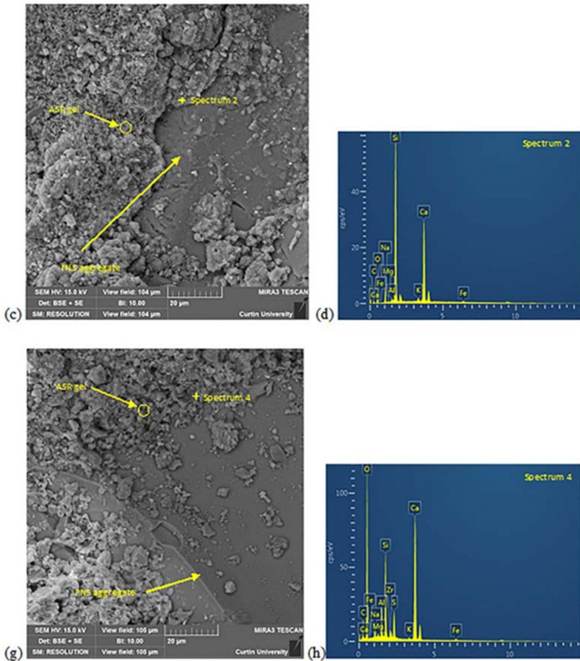
**Figure 8** SEM and EDS of specimens after 21 days of NaOH exposure
