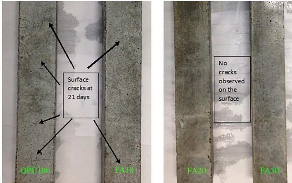
**Figure 6** Visual inspection of AMBT samples after 21 days exposure
