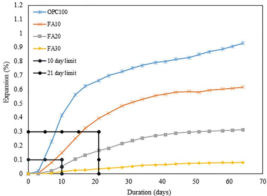
**Figure 5** ASR expansion of mortar bars containing different percentages of fly ash
