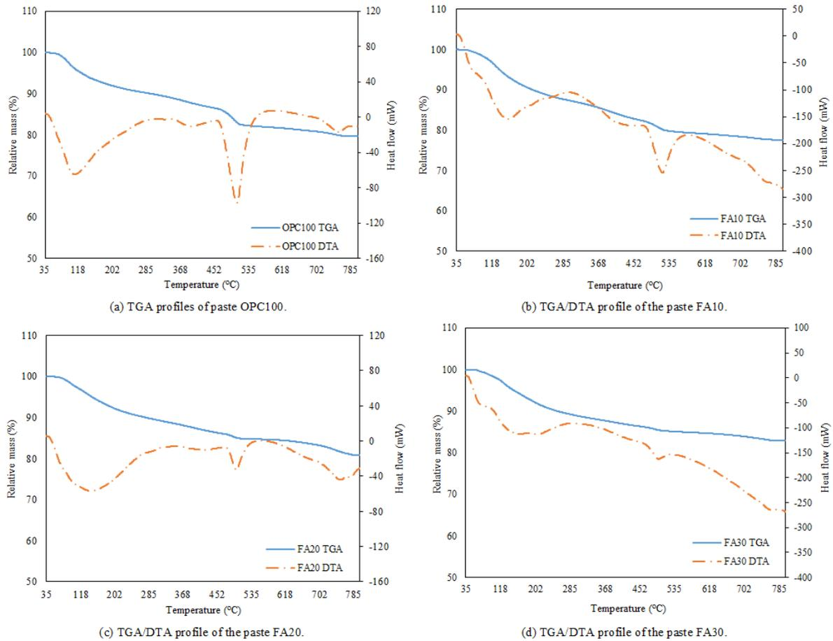
**Figure 7** Thermogravimetric mass changes of paste samples exposed to AMBT condition
