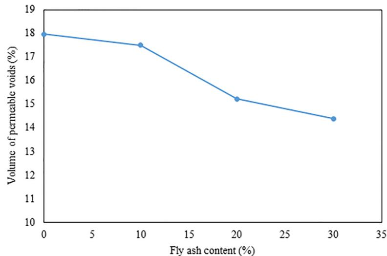
**Figure 4** Volume of permeable voids of mortar with respect to fly ash percentage
