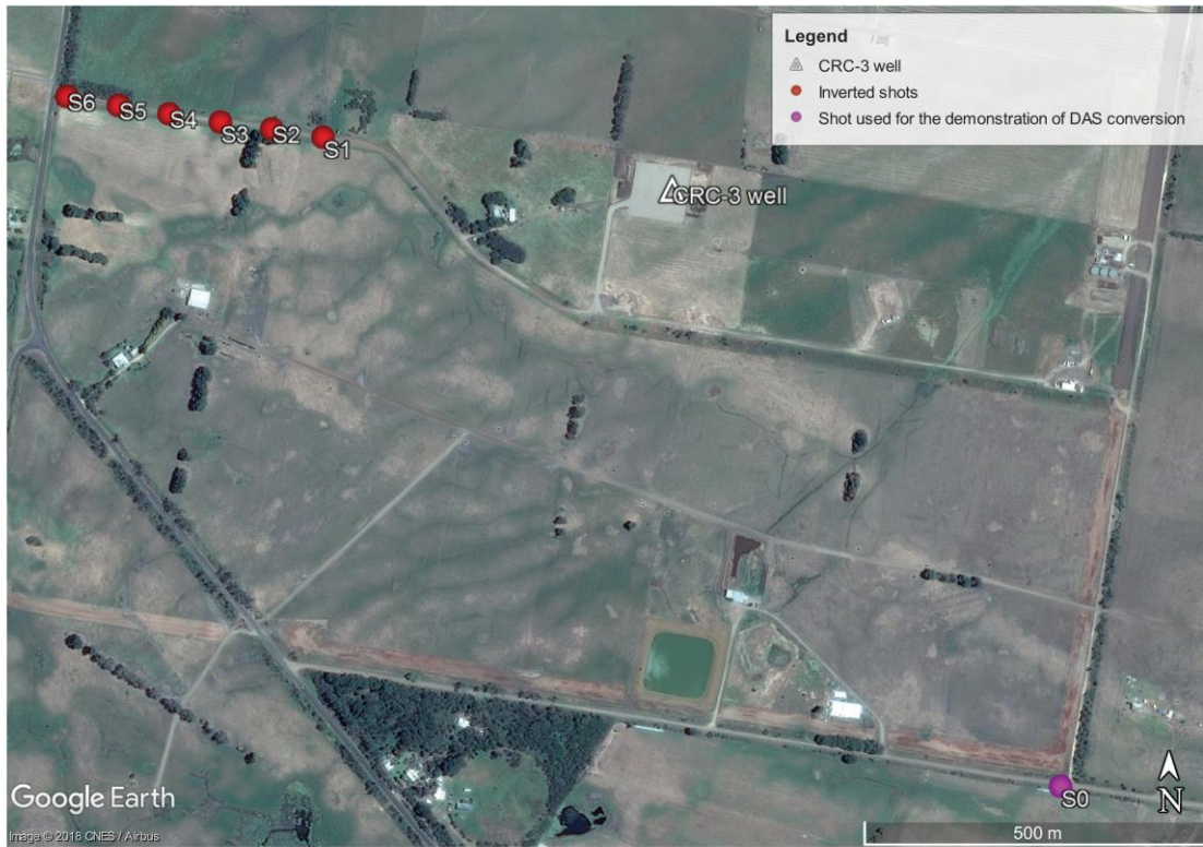
Figure 1. Map of the survey site: shot points used for the inversion (red) and the shot point used to demonstrate DAS conversion (purple).
