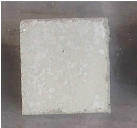
Fig. 6 (a) PC-FNS100 before wet–dry cycles and (b) PC-FNS100 after wet–dry cycles.
