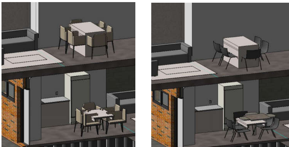
Figure 2.9 Example of how a chair as a 3D object makes changes to a project
