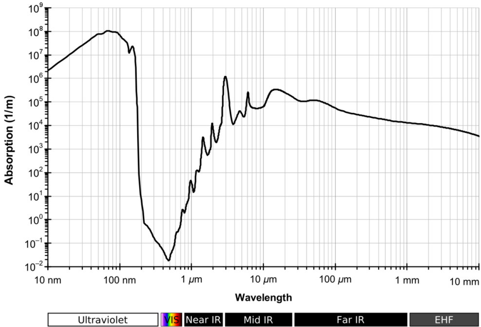
Figure 1.2: Liquid water absorption spectrum across a wide wavelength range.
