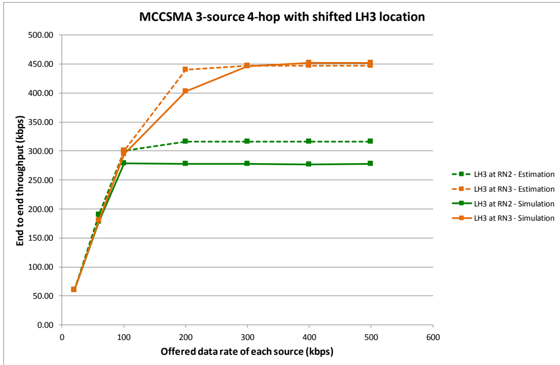
Figure 4-30 Comparison between estimation and simulation for 3-source 4-hop shifted LH3 location with MC CSMA protocol
