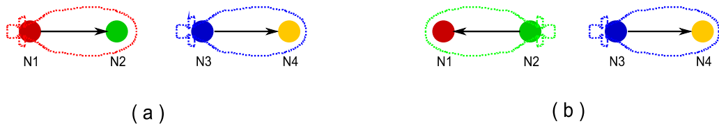
Figure 2-7 Examples of directional antenna radiation patterns aimed at reducing the effects of (a) hidden node, and (b) exposed node problems.
