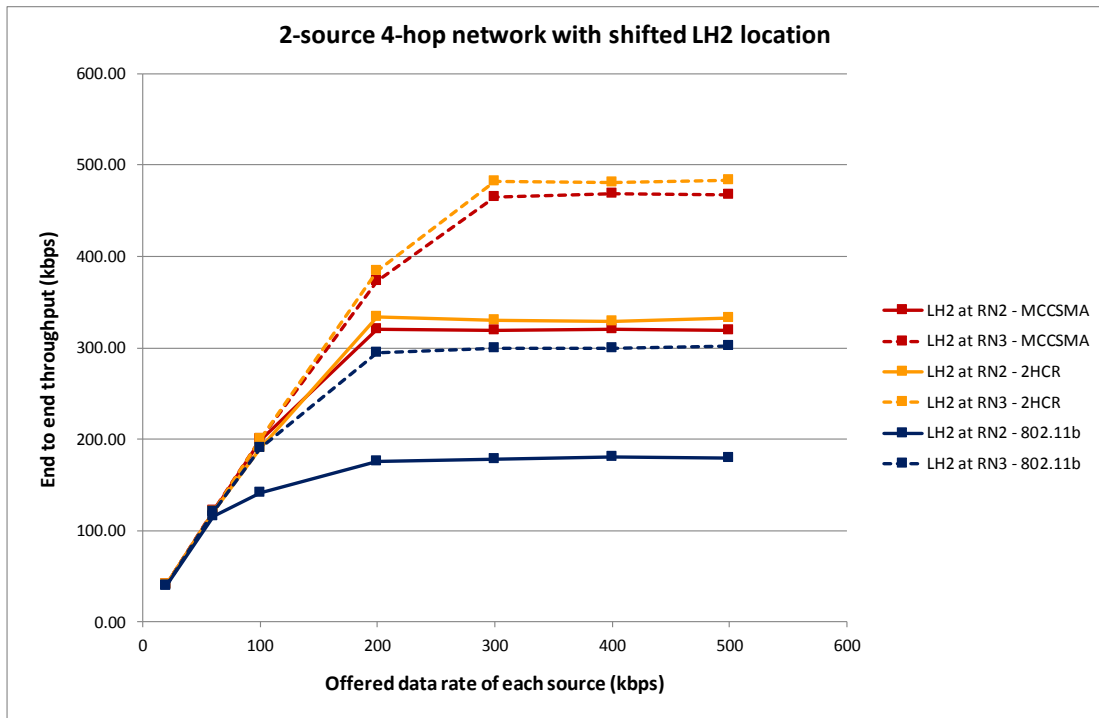
Figure 3-15 The end to end throughput of 2-source 4-hop networks with shifted LH2 location
