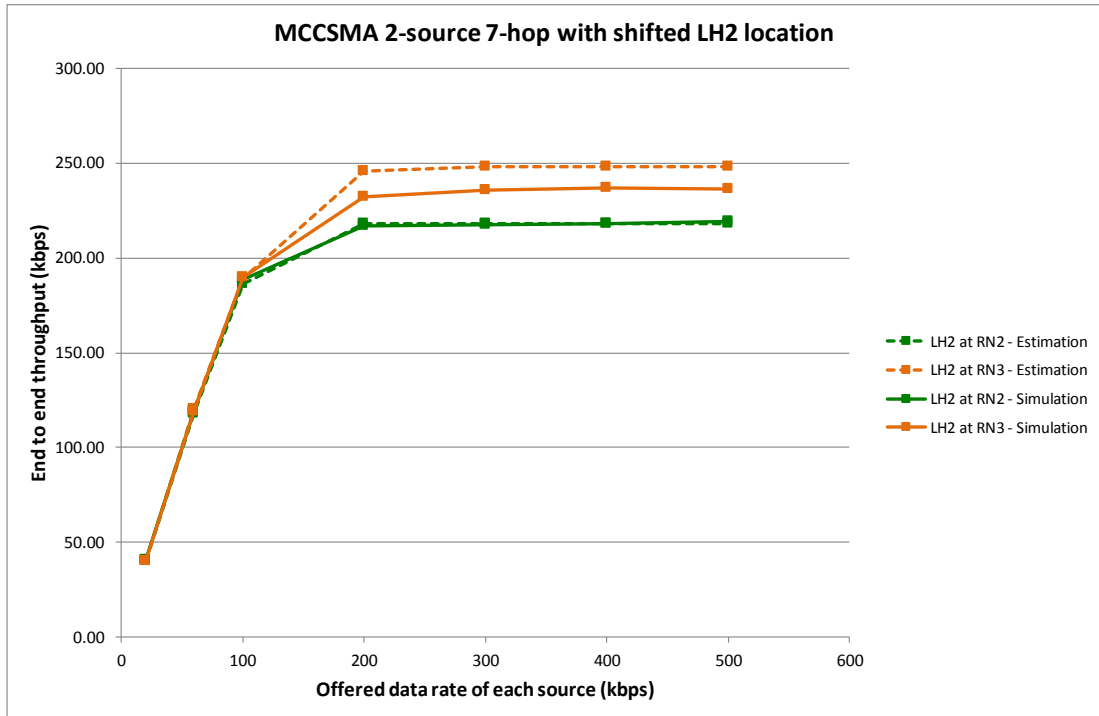
Figure 4-31 Comparison between estimation and simulation for 2-source 7-hop shifted LH2 location with MC CSMA protocol
