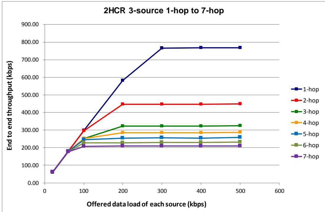
Figure 4-8 The end to end throughput of 3-source multihop networks with 2HCR protocol
