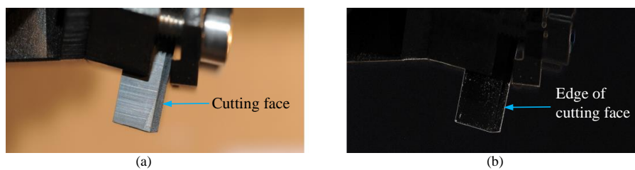
Fig. 11: (a) Photo of a blunt cutter, and (b) blunt cutter edges (ImageJ software).
