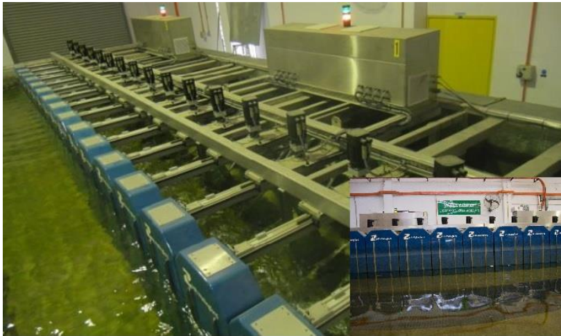
Figure 3.4: H R Wallingford Wave Maker
