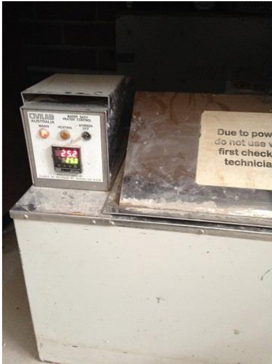
Figure 4-30: Water bath used for testing soil density.
