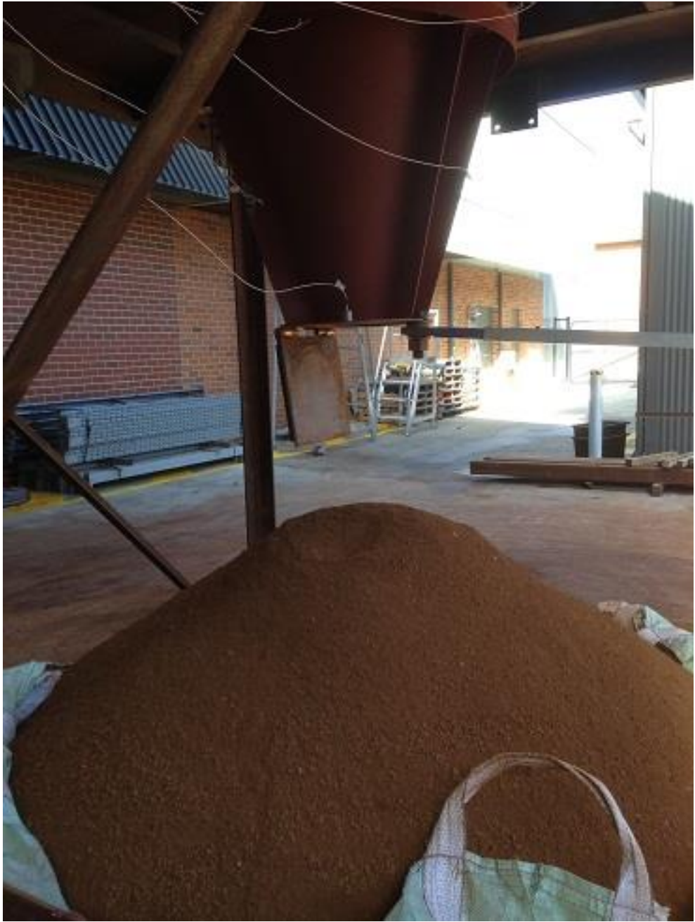
Figure 4-10: 200 mm hopper opening with swing gate open.
