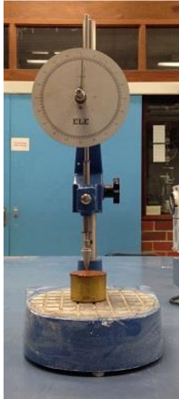
Figure 4-28: Apparatus to test soil liquid limit.
