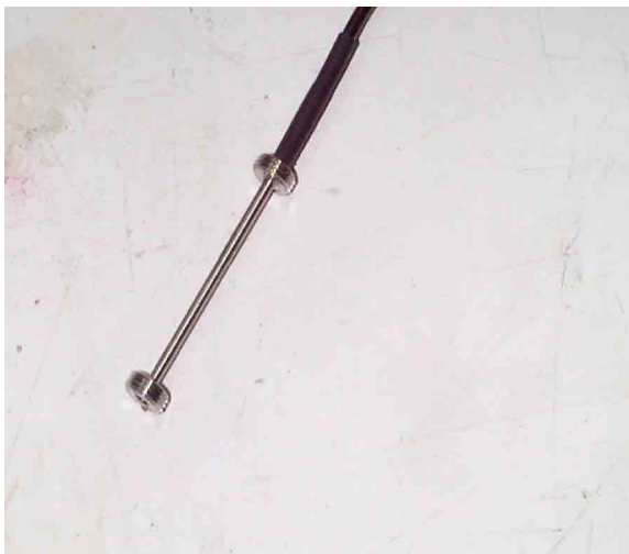
Fig. 4 Fiber optic strain sensor.
