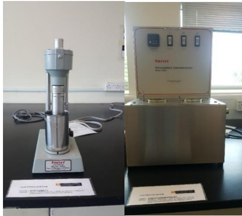
Figure 3-4: Fann viscometer (left) and Fann atmospheric consistometer (right)
