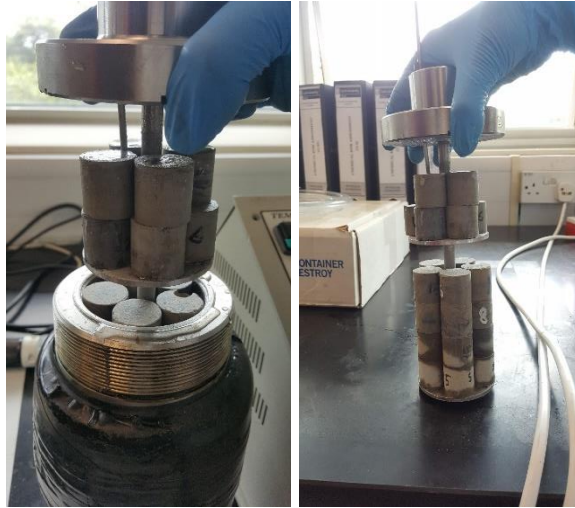
Figure 6-4: Samples after exposure to water saturated scCO 2
