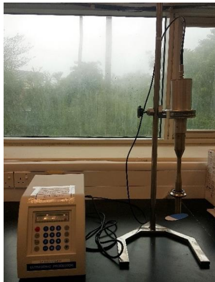
Figure 3-14: LSP-500 Laboratory-Scale Processor used for the dispersion of NS
