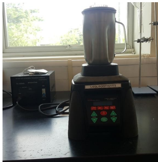
Figure 3-2: Fann constant speed mixer used for the purpose of this study
