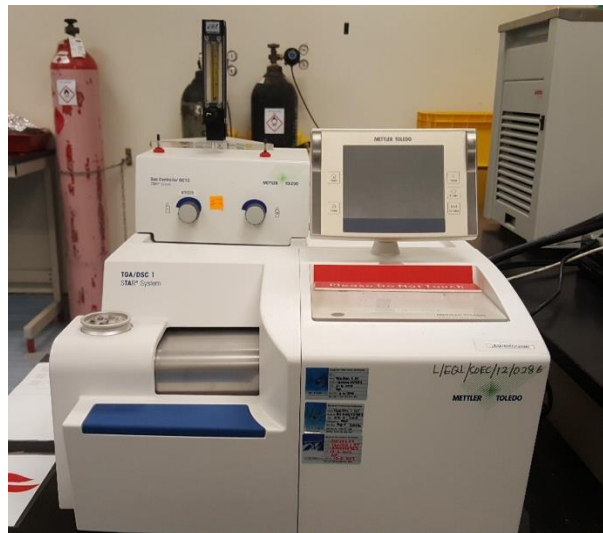
Figure 3-12: Mettler Toledo Thermo Gravimetric Analysis (TGA) used for the material characterization
