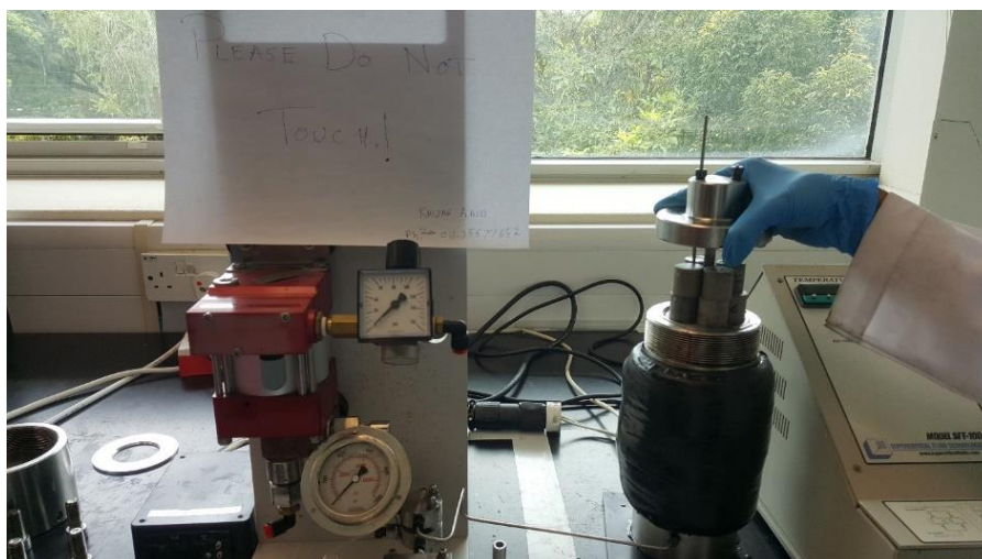
Figure 6-3: Static reactor used to expose the cement samples to water saturated scCO 2 for 40 days
