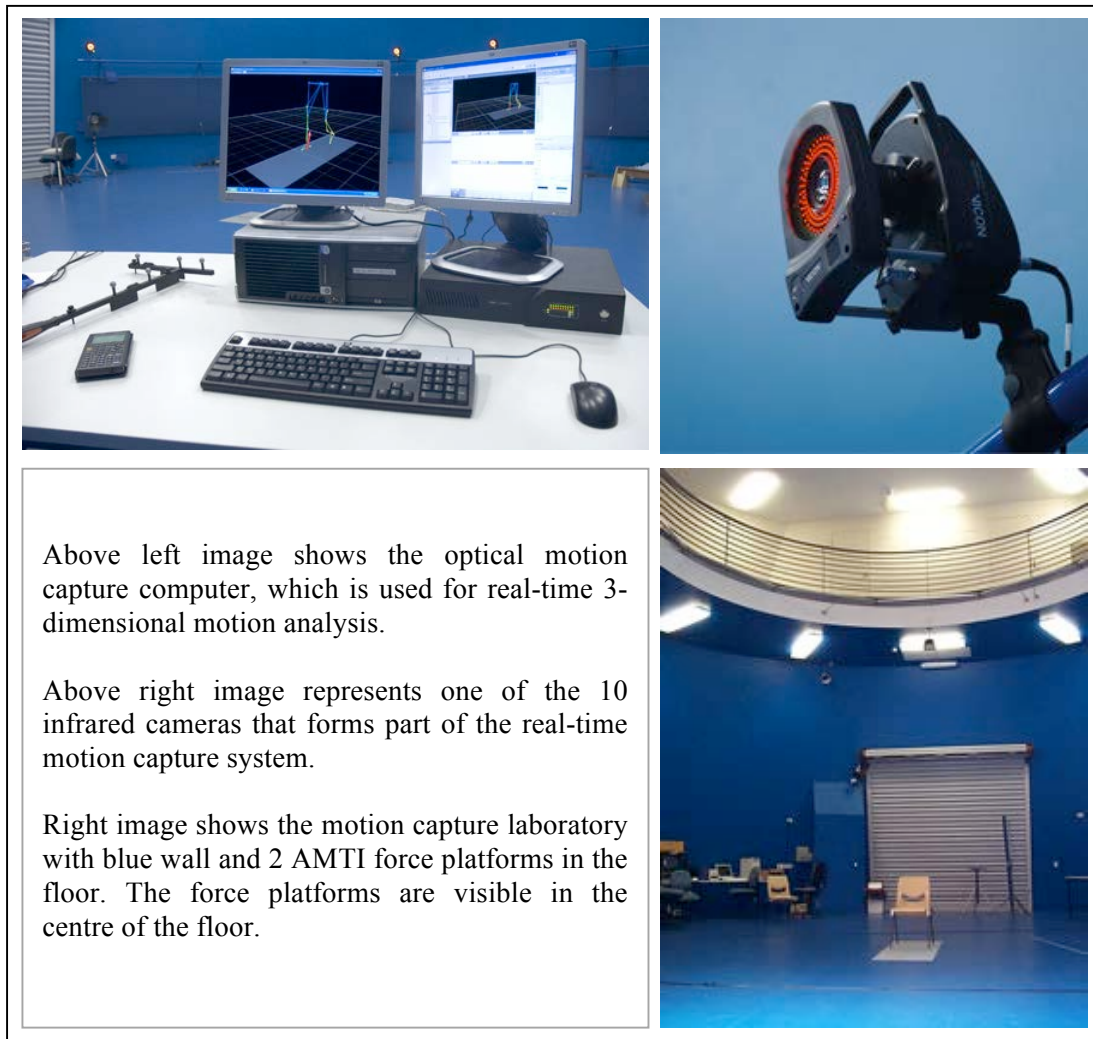
Figure 9. 1. The main laboratory apparatus of the Motion Capture Technique. Source: Curtin School of Physiotherapy, n.d.
