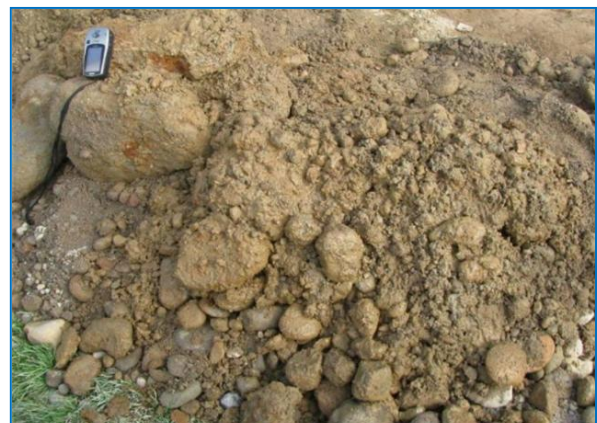
Fig. 6 Cobbles and boulders collected during the excavation
