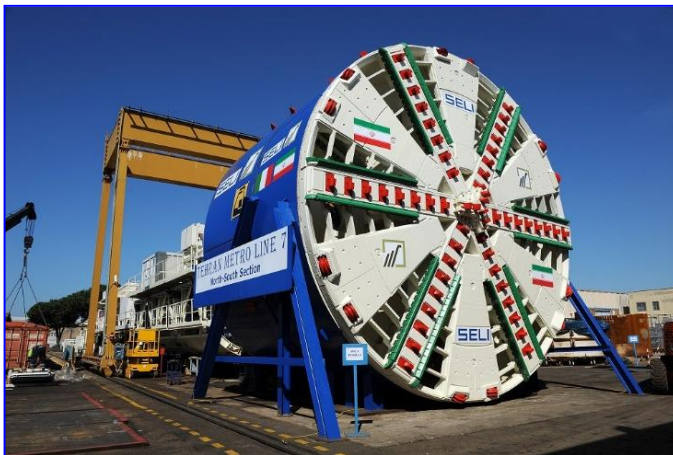
Fig. 3 General view of the North-South Lot of Tehran Metro Line 7 EPB-TBM
