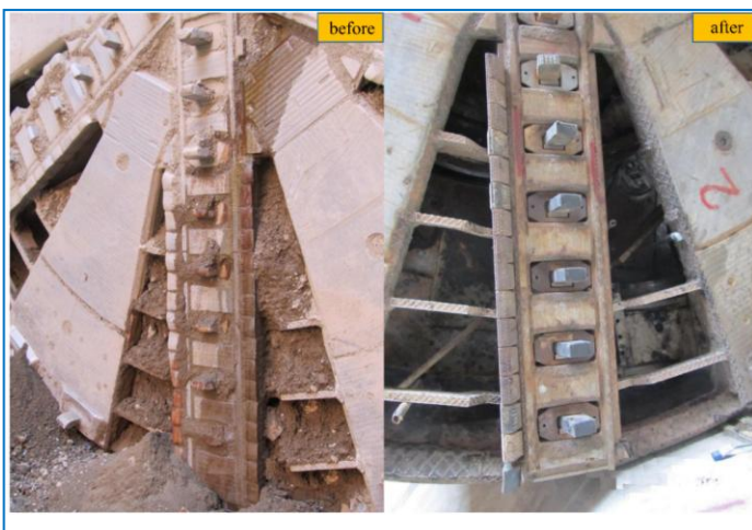
Fig. 7 Cutting tools before replace showing wear (left) and after replace (right)
