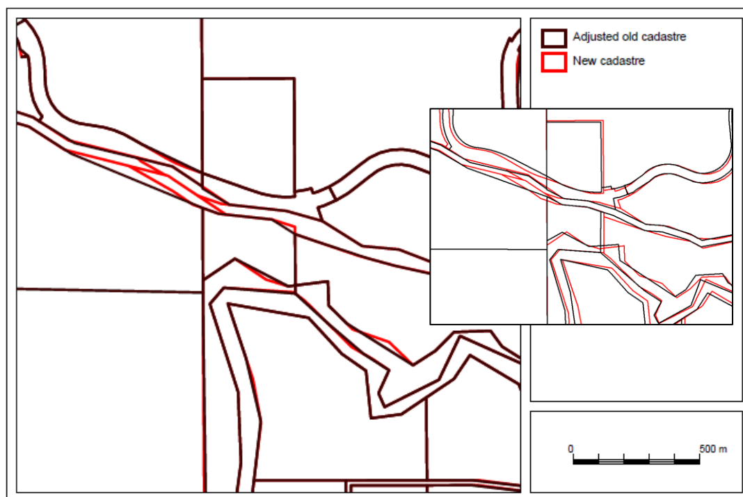
Figure 8.4 Several clearly revealed adjustment failures
