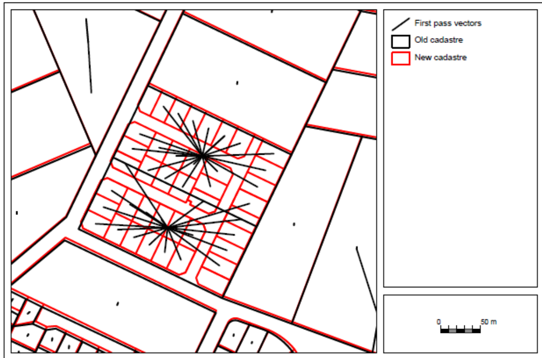
Figure 4.24 An area with a new subdivision
