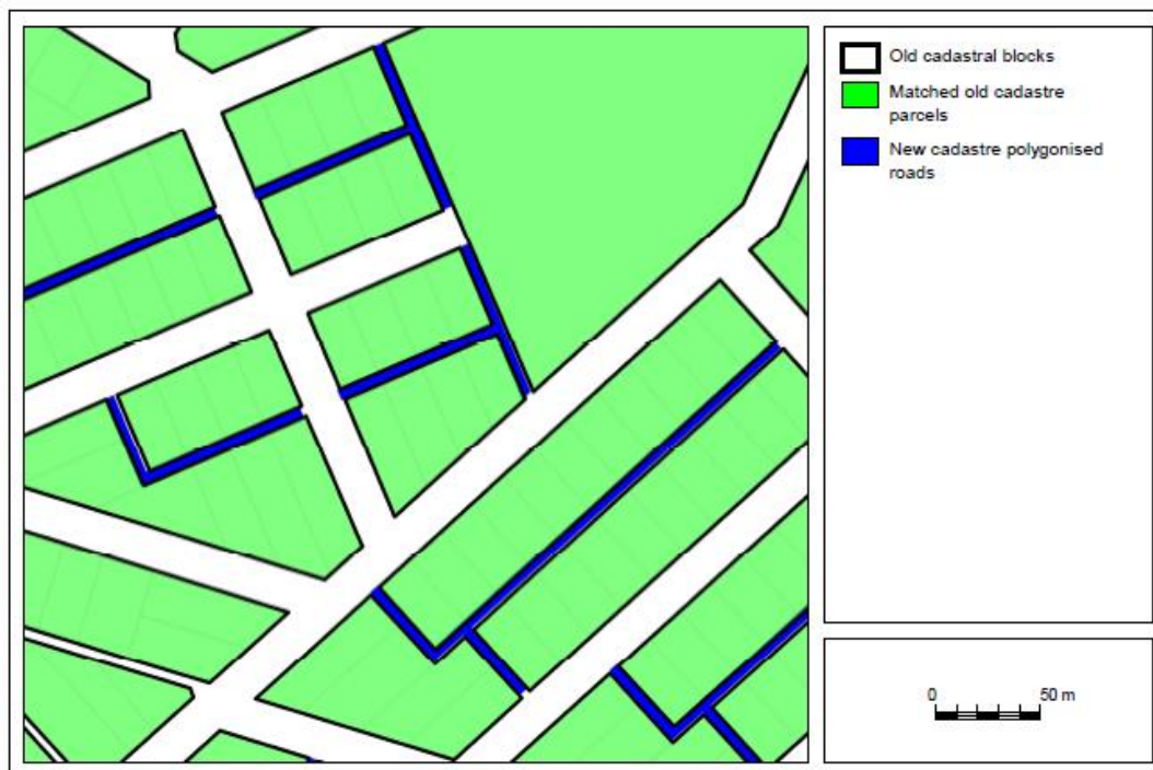
Figure 4.2 An area where several roads are modelled as polygons in the new cadastre but not in the old.
