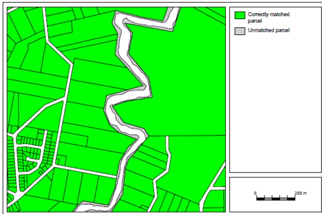
Figure 4.8 An area that includes a section of creek where the parcel boundaries do not follow the creek boundaries
