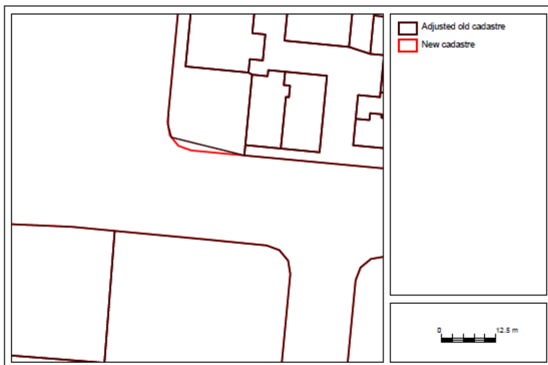
Figure 6.8 Poor adjustment due to an incorrect boundary match
