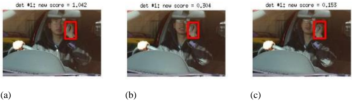
Figure 5.8 : Similar looking proposed regions with different detection scores
