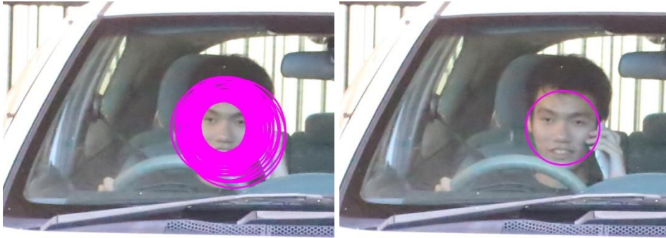
Figure 4.15 : Images show face detection as indicated by coloured circles when minNeighbour is set to 0 (left) and when minNeighbour is set to 2 (right)
