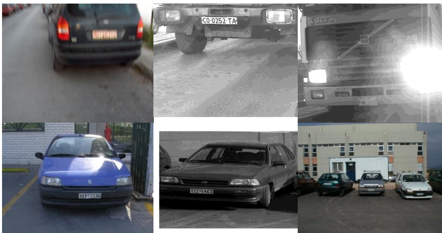
Figure 3.4 : Examples of undetected LP positive images from a variety of difficult positive image data subset
