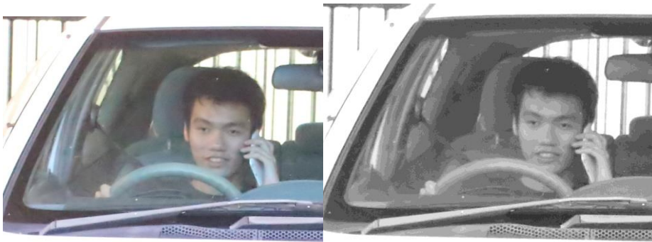
Figure 4.13 : Coloured (left) to grey scale (right) image conversion
