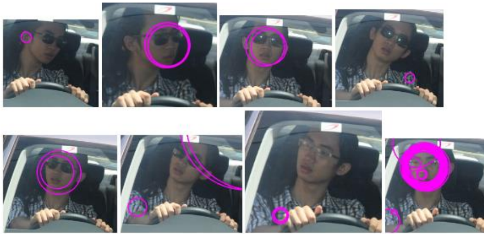
Figure 4.25 : Various levels of face angle affecting face detection performance
