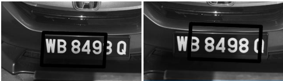
Figure 4.21 : Differences in LP detection bounding boxes due to slight lighting variation
