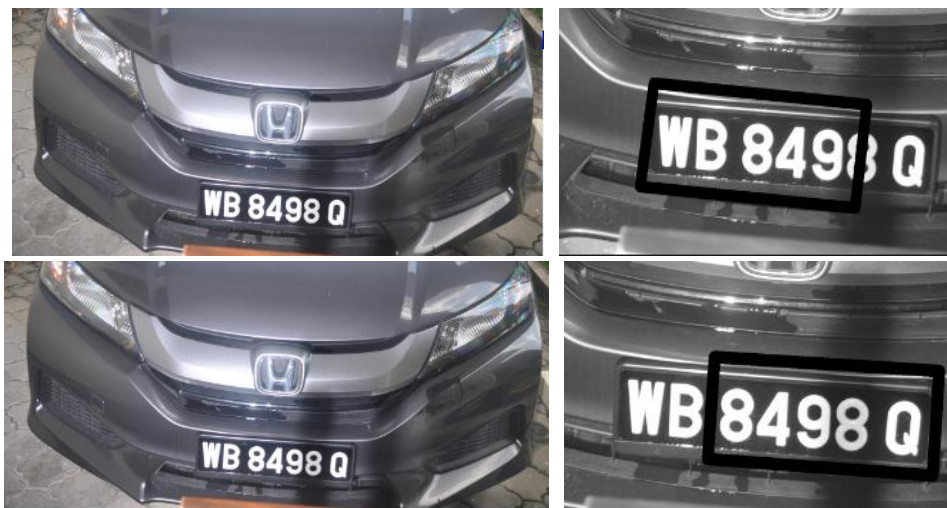
Figure 4.22 : A subtle lighting variation which resulted in dissimilarities in LP detection predictions
