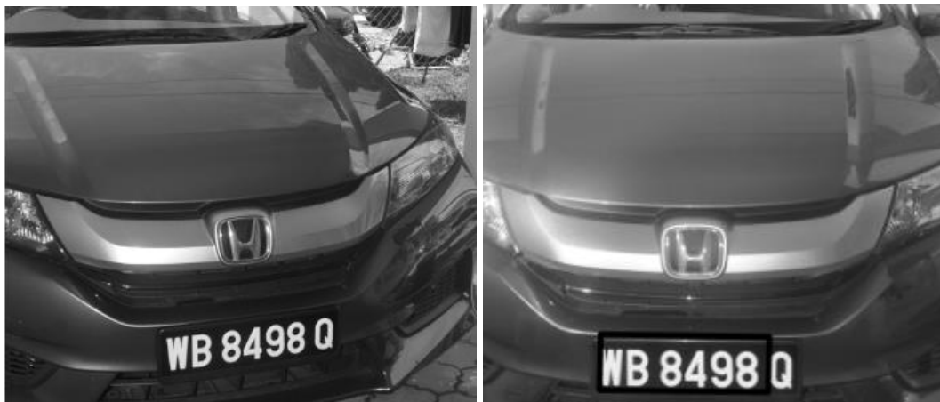
Figure 4.24 : The left image depicts an undetected LP in an image taken at an angle to the vehicle front whereas the right image shows LP detection in an image captured from a perpendicular angle to the vehicle front
