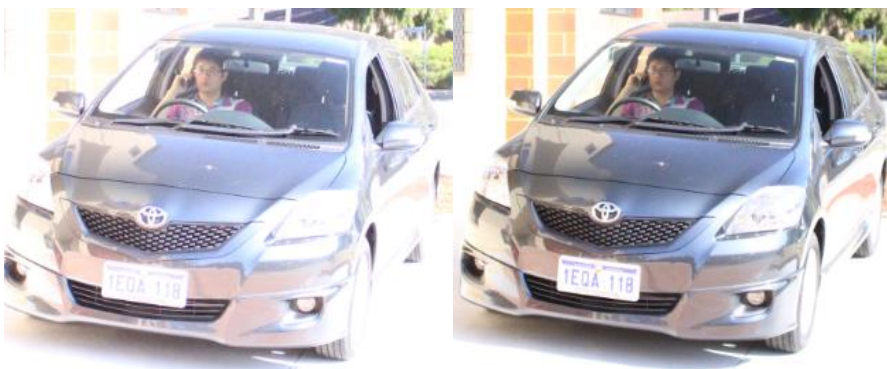
Figure 4.2 : Glare on vehicle windshield (left) reduced by polarizing lens (right)
