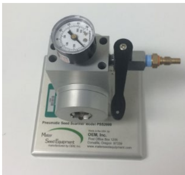
Figure 2.3. Pneumatic seed scarifier (Model PSS2000, OEM, Inc.) Used for mechanical scarification of Eragrostis eriopoda and Fimbristylis dichotoma seeds.
