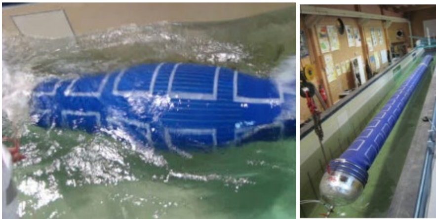
527 528 Figure 19: EAP Generator (SBM, 2019) 529
