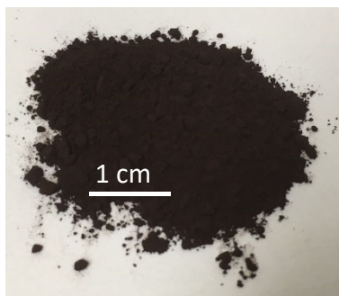
Figure 4-2. Nanopowder (bare MNPs) as received from the manufacturer
