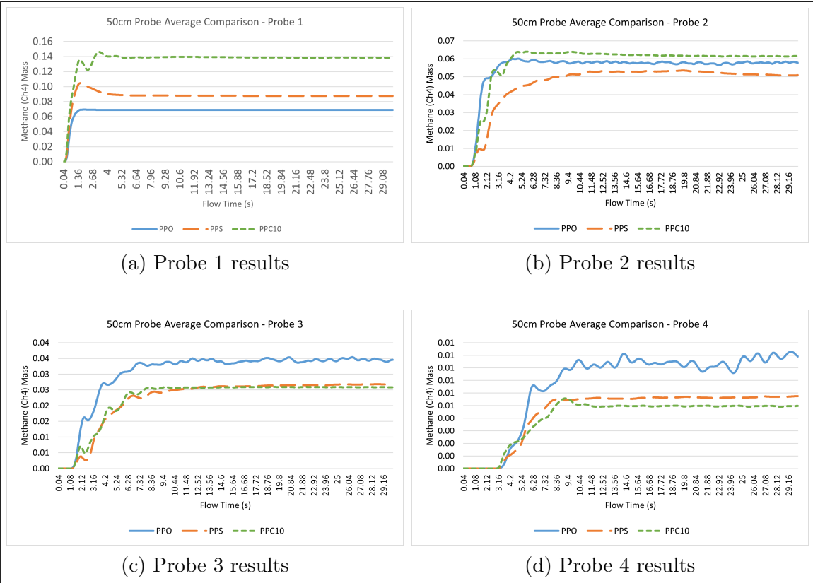
Figure 4.9: Graphed values from the methane probes. PPO represents the Pan Pipes Original geometry, PPS Simplified and PPC the 10cm Cubified variant.
