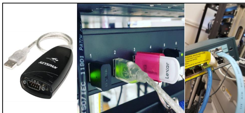
Figure 5-29 - Keyspan USB to Serial Adaptor (Left)- Keyspan USB connection to AnyConnectUSB Hub (Middle)- Console connection to WLC (Right)
