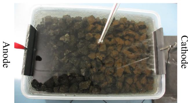
Figure 9. Brown precipitate produced in the process of coal modification.
