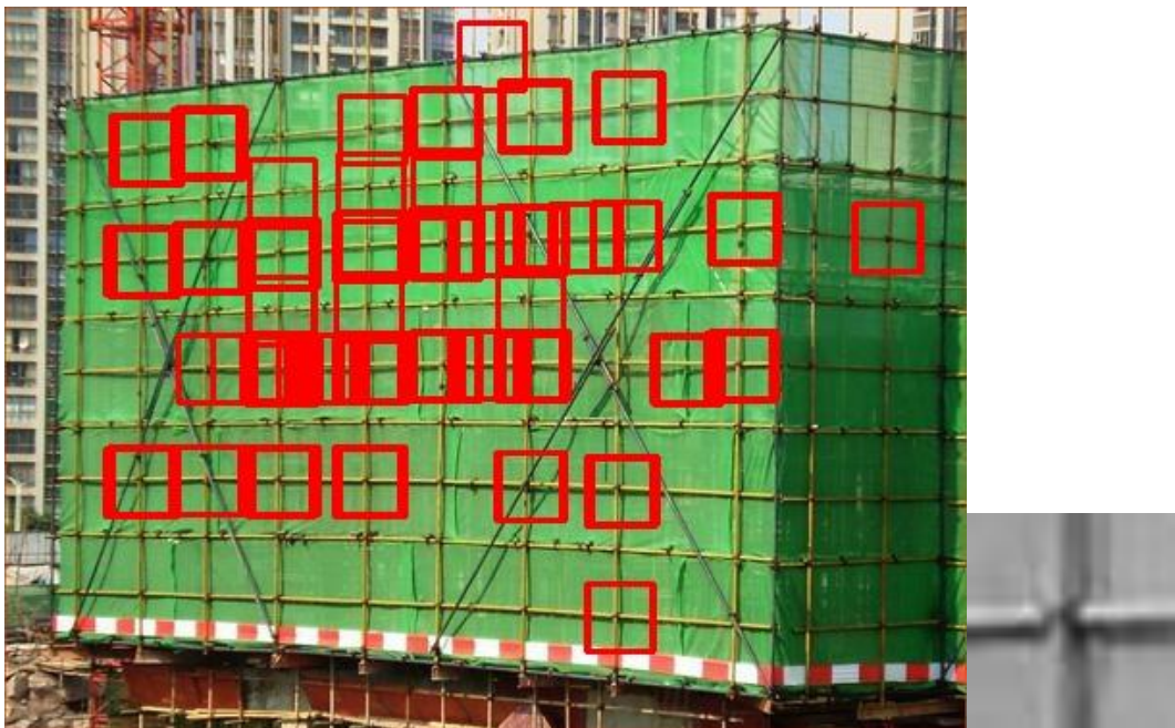
Figure 5.11(d). The detection result of TM with the template photo on the right
