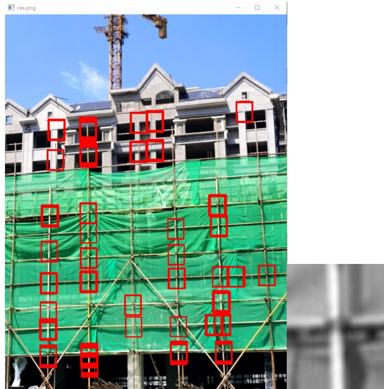
Figure 5.13(d) The detection result of TM with the template photo on the right
