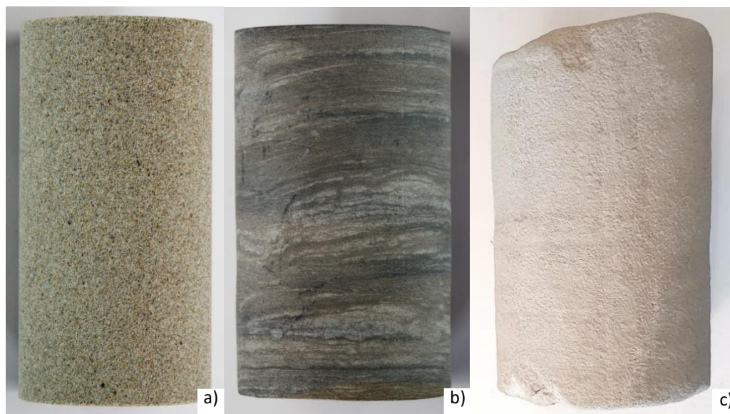
Figure 7.3: Formation cores used in wettability test. a) Berea sandstone core, b) Shale core, and c) Malaysia sandstone core
