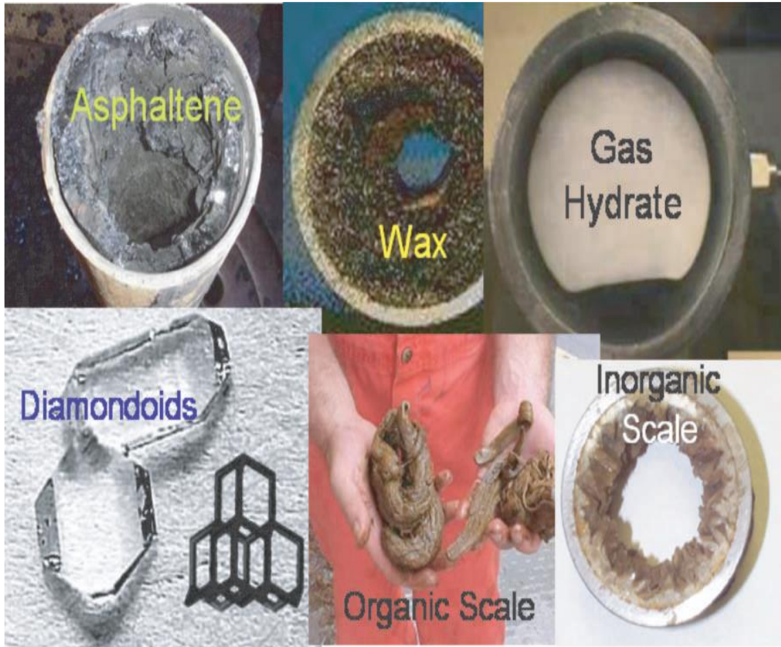
Figure 1.1. Different types of solids formed obstructing the flow in pipelines. (Reproduced from (Mullins, 2007) with permission from Springer Nature)
