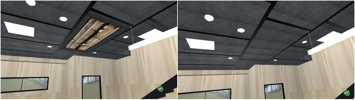
Figure 5.23 – Acoustic felt ceiling panels reveal insulation and allow access to mechanical and electrical plant services throughout the multiple lifecycles of the building.
