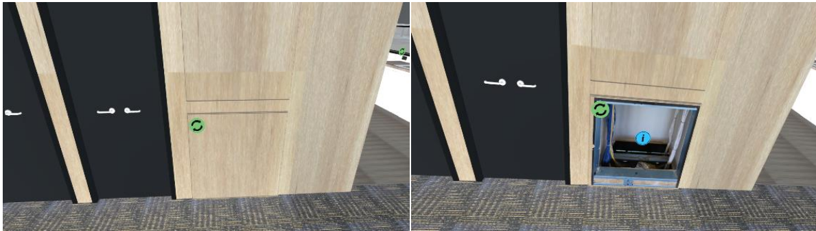
Figure 5.22 – (a) Wall panelling hides the service duct connecting the roof space to the first floor and ground floor ceiling. (b) VR model exposes the lower access panel, revealing the service duct.
