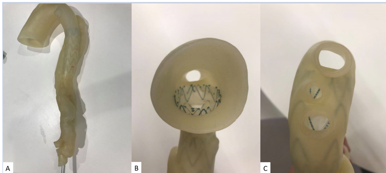
Figure 3. Stent graft deployed in 3D printed model. The aortic model was printed with Visijet CE-NT A30. (A): Deployed stent graft visible through model wall. (B): Axial view from proximal aortic arch. (C): Caudal view down aortic arch vessels. Reprinted with permission under the open access from Wu et al. [25].
