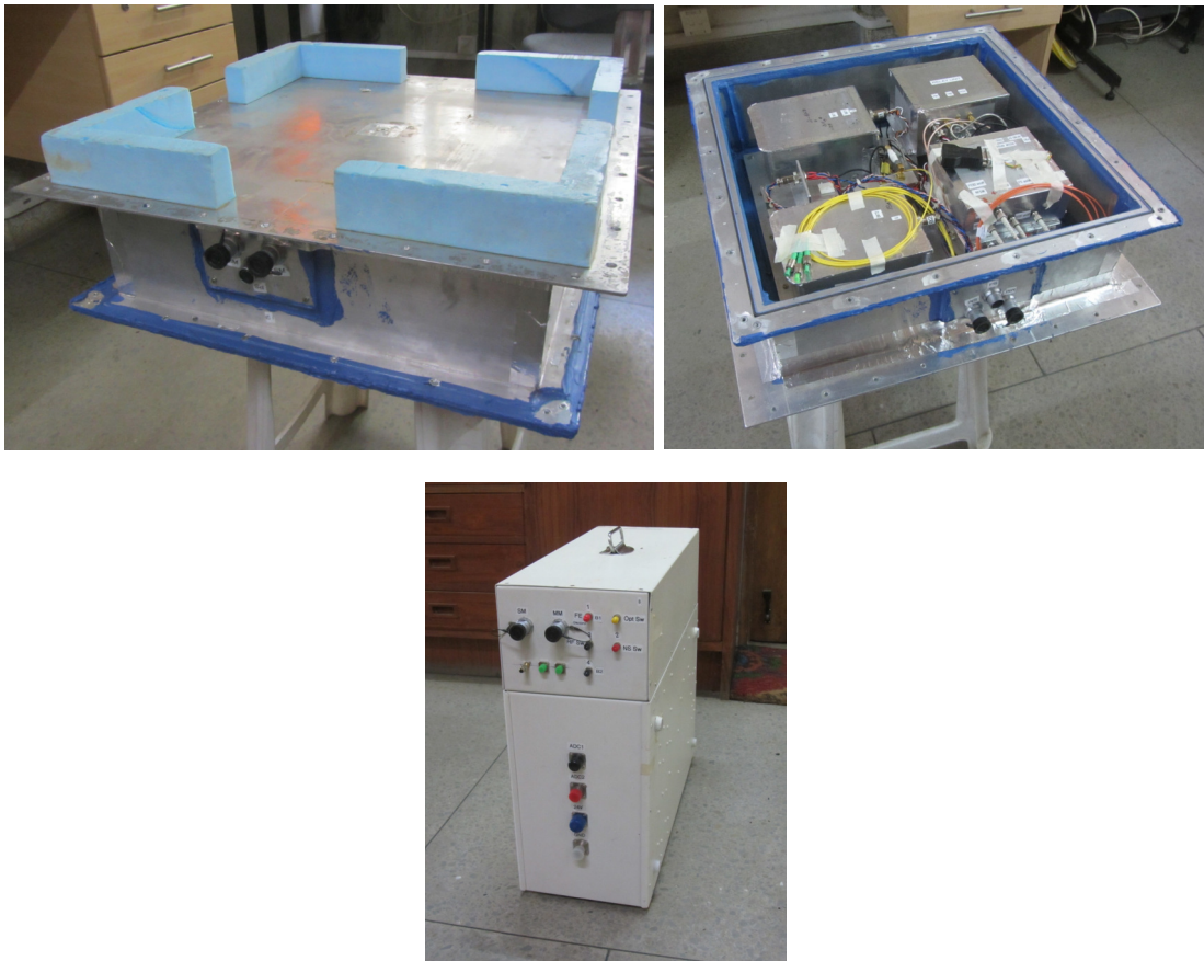
Figure 3.4: The analog electronics enclosures beneath the antenna and at the remote base station. In the top panel on the left and right are shown the enclosure at the antenna base; the left panel shows its view from the top and in the right panel is shown the view from below with the bottom cover removed. The bottom panel shows the enclosure that houses the analog electronics at the remote station.
