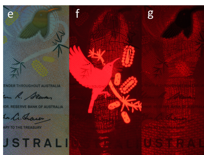
Figure 3. (a,c,e) Unilluminated and (b,d,f) illuminated at 350 nm and (g) 450 nm charged latent fingermarks (one female donor) deposited on Australian polymer banknote. The illuminated marks were pictured through a deep red filter. The marks were shaken at 20 rpm for 20 min in a MPA-coated CIS-ZS QDs solution. See ES1+ and Table S1 for the photography details.
