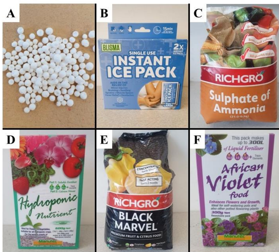
Figure 4.1: Sources and precursors used to prepare AN: (a) explosive grade AN, (b) AN based cold packs, (c) commercial ammonium sulfate fertiliser, (d) hydroponic nutrient product containing calcium nitrate, (e) Black Marvel fertiliser containing 11.7% w/w \text{NH}_4 and (f) African Violet Food containing 10.5% w/w \text{NH}_4 .
