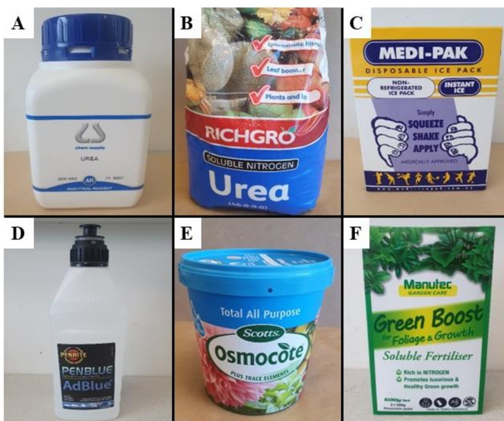
Figure 5.1: Urea products used to prepare UN: (a) chemical grade urea, (b) fertiliser urea, (c) cold pack urea, (d) DEF, (e) Osmocote fertiliser mixture, (f) Green Boost fertiliser mixture.
