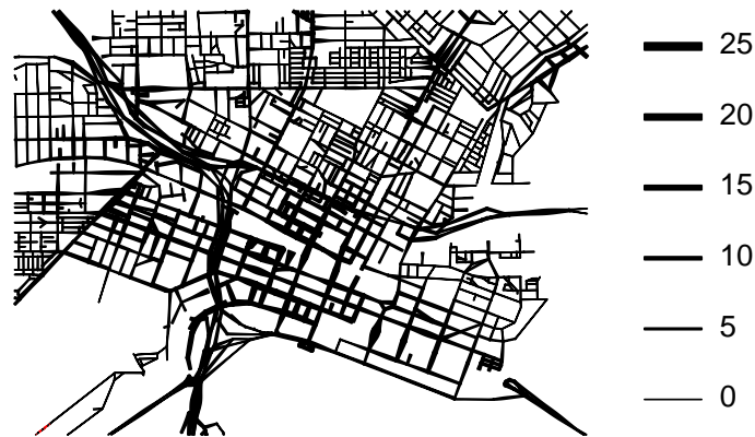
Figure 11: Kernel estimate of accident intensity for Perth CBD, using Euclidean kernel with fixed bandwidth 91 metres selected by leave-one-out cross-validation. Uniform correction (20). Line thickness proportional to intensity values.
