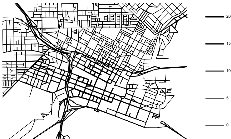
Figure 10: Estimate of traffic accident intensity in the Perth CBD using the heat kernel algorithm with bandwidth 330 metres. Intensity values (accidents per km per year) proportional to line widths.
