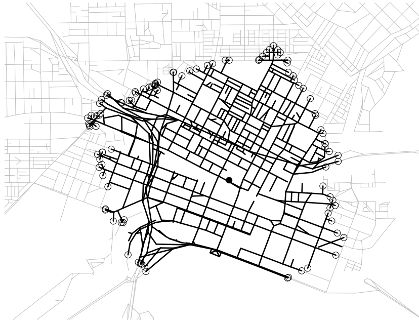
Figure 9: A “disc” of radius r = 2 km in the Perth CBD road network defined using the shortest-path distance metric. Filled circle: centre point u . Thick lines: disc d_L(u, r) . Open circles: points counted in the circumference m(u, r) .
