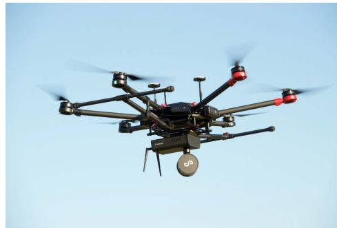
Figure 2.3 Emesent's Hovermap Mining payload (Hovermap, 2019)
