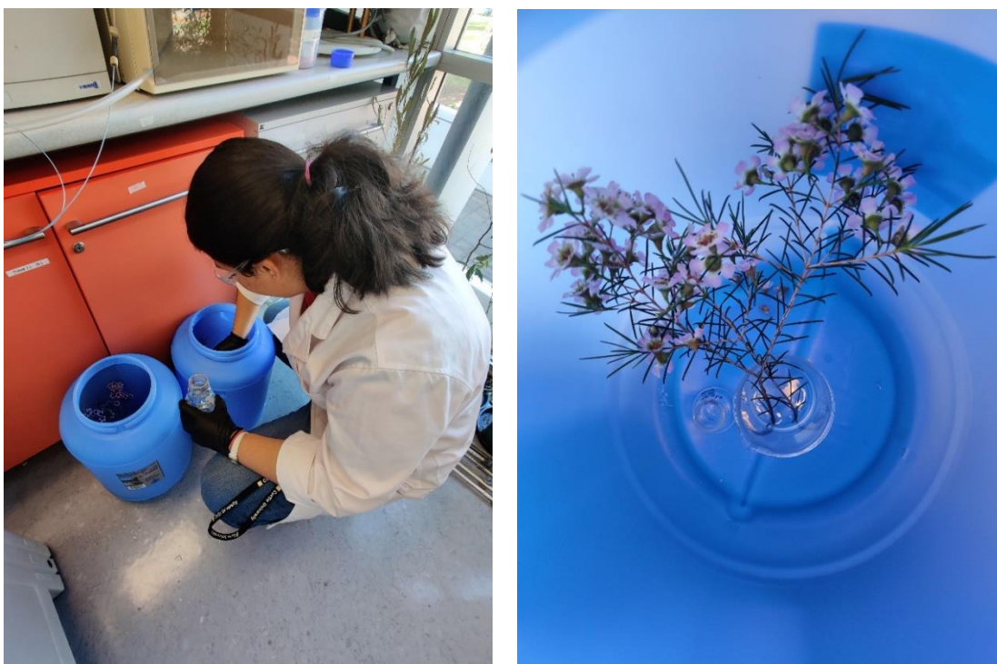
Figure 20: 25 L containers being filled with Geraldton wax and ethylene solution/procedural blank solution (left) Geraldton wax places in flask with ethylene/procedural blank solution placed next to it (right).
