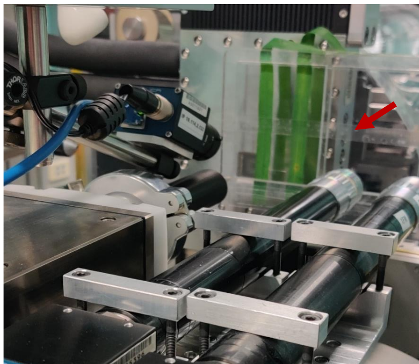
Figure 16: Visualisation of 2D MAIA Synchrotron XFM setup with whole wheat leaf samples, red arrow indicating direction of x-ray beam
