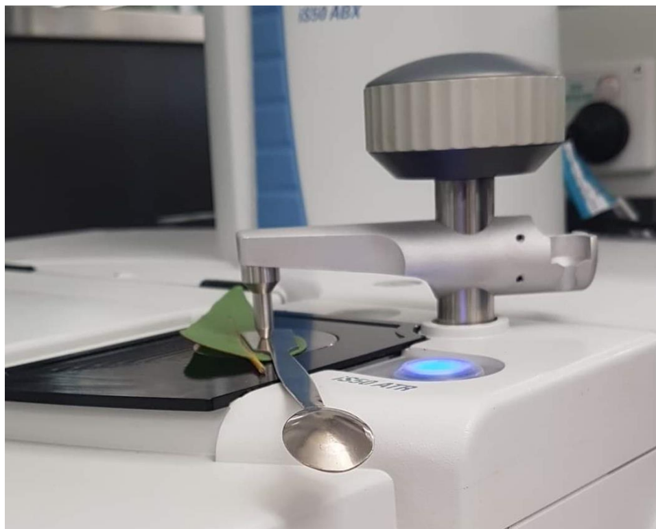
Figure 24: Spatula implemented between pressure arm and sample utilised for eucalyptus ATR analysis.
