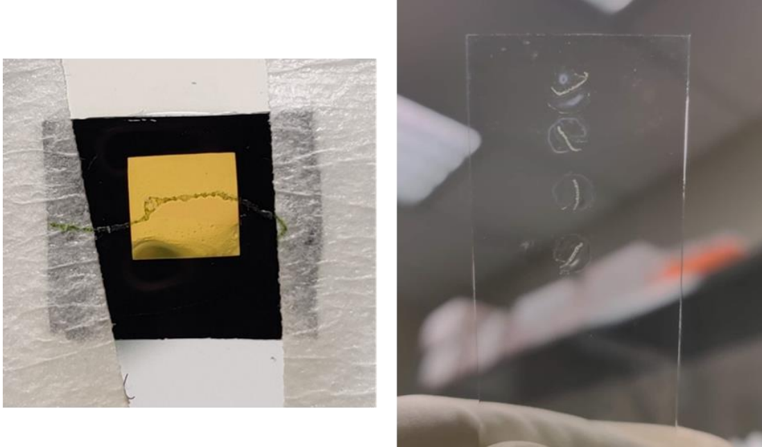
Figure 23: tissue sections of wheat on silicon nitride chip (left) and microscope slide (right)
