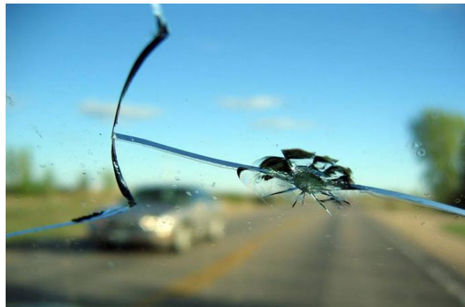
Figure 3-11 - Crack propagation is arrested at pre-existing discontinuities. (Cal Auto Glass, 2016)
