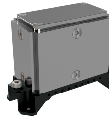
Figure 5: A render of the shielding surrounding the radiation detection payload.
