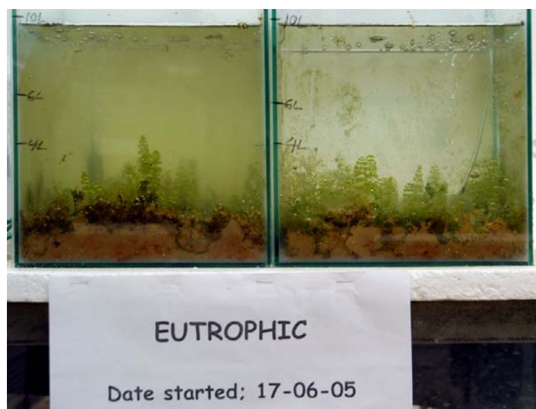
Figure 6.4 Nutrient enrichment - the eutrophic set-up. The eutrophic treatment consisted of N. congesta culture enriched to a total phosphorus concentration of 100 \mu\text{gL}^{-1} (four replicates) for 136 days.
