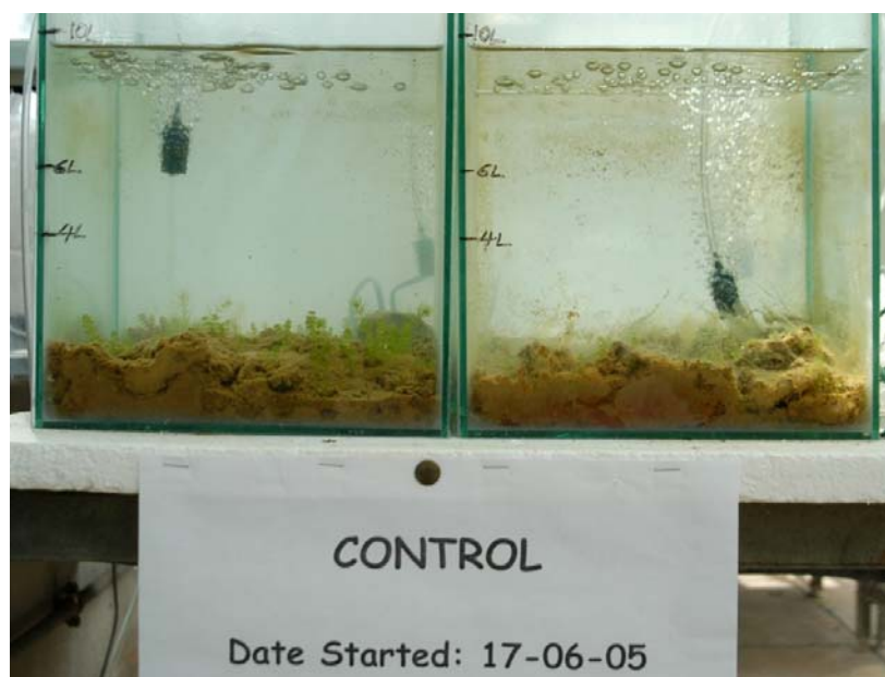
Figure 6.2 Nutrient enrichment - the control (oligotrophic) set-up. The control treatment consisted of N. congesta culture without phosphorus enrichment (four replicates) for 136 days.
