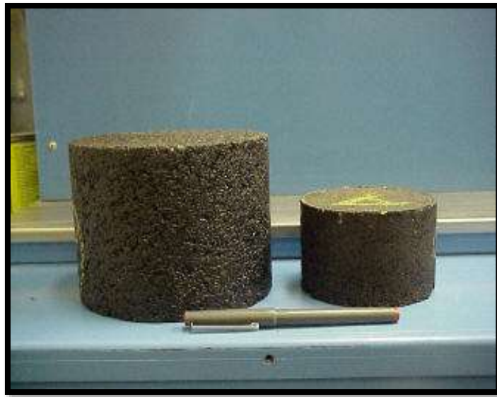
Figure 41: SuperPave compactor sample (left) VS. Marshall Compactor sample (right)
