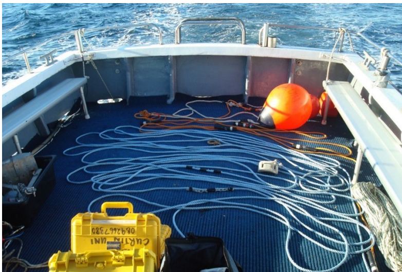
Figure 4-9: Retrieve float and line prior to deployment
