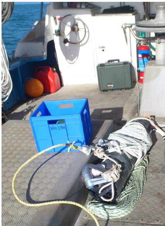
Figure 4-40: Recorder (left) and retrieve line and buoys (right) ready for deployment
