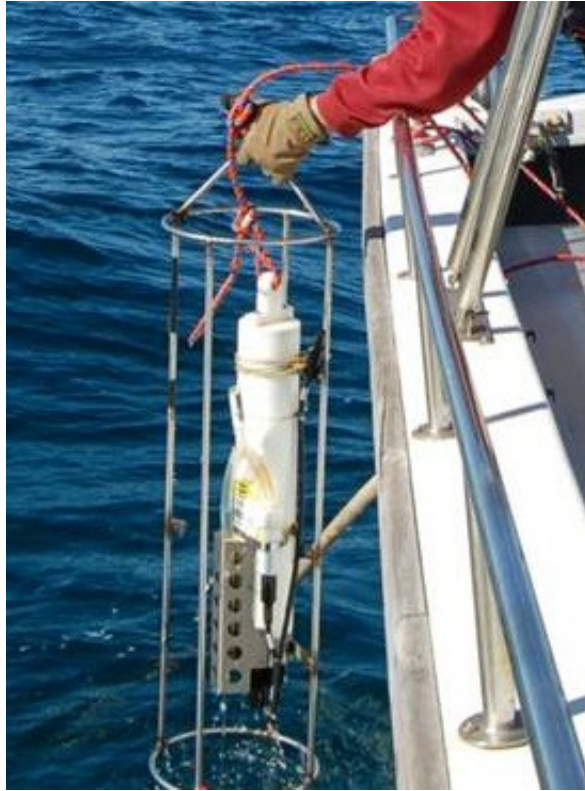
Figure 4-13: Seabird SBE 19 Plus Conductivity, Temperature, Depth Probe
