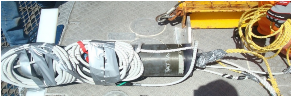
Figure 4-8: Receiver high pressure housing with excess cable (image from deck of L3 trial)
