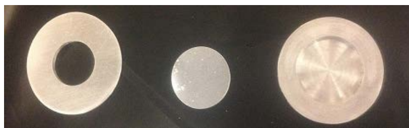
Figure 4.3 Zinc foil target that is contained between an aluminium target annulus (left) and an aluminium cradle (right).
