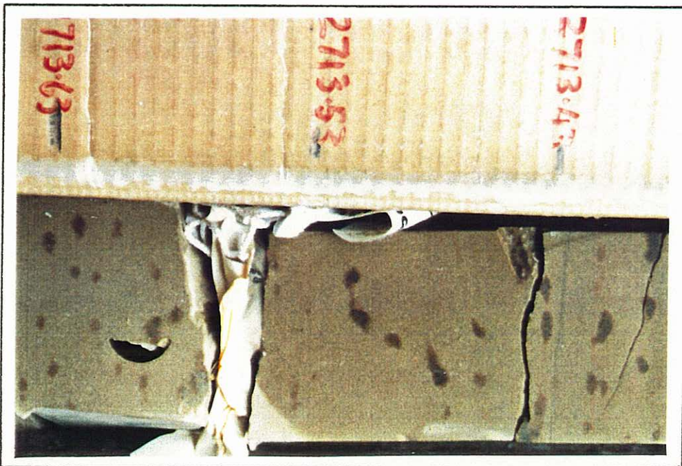
Figure 34. Photo of Bambra-1, core 2, 2713.4-2713.65m displaying sideritised horizontal worm burrows within very weakly planar laminated fine grained sandstone.
