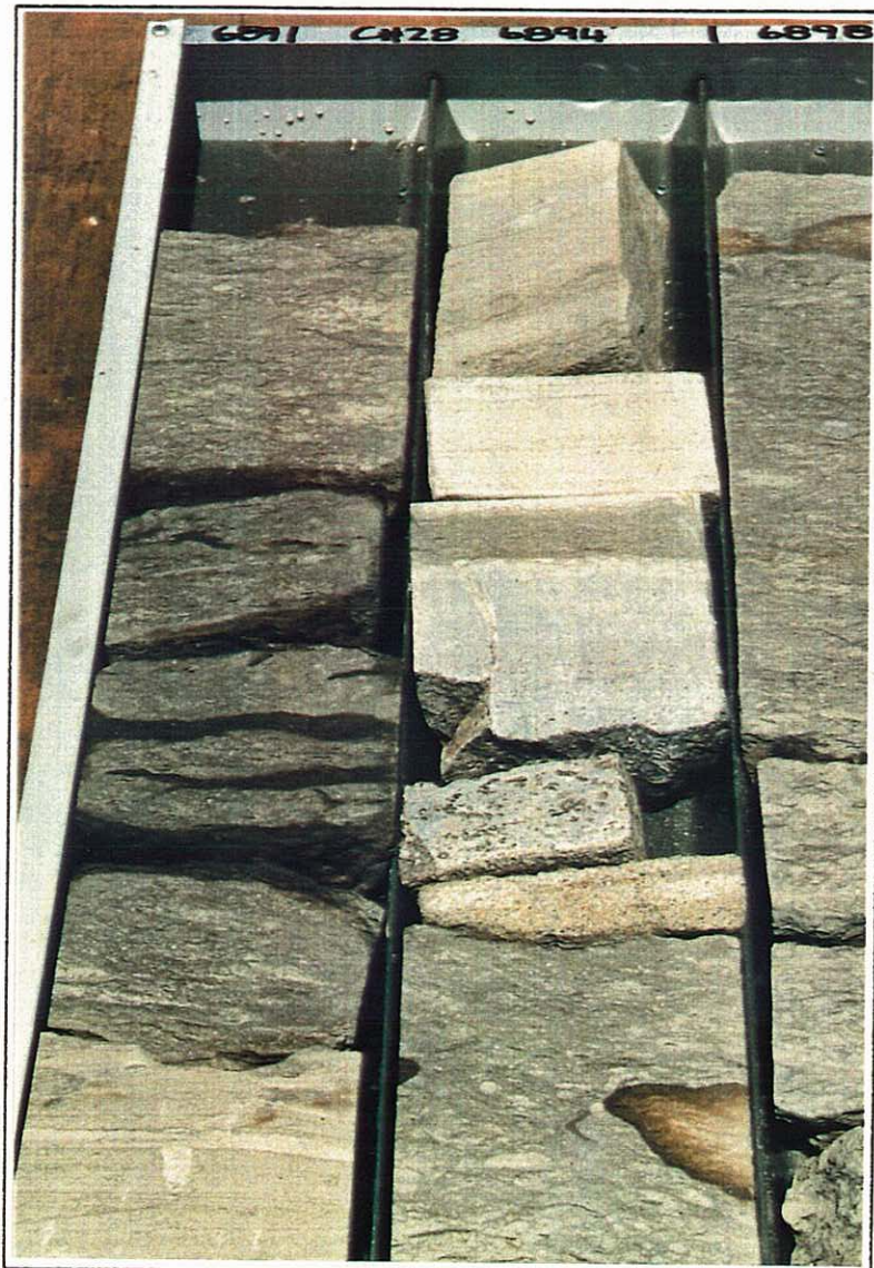
Figure 40. Photograph displaying interbedded relationship of facies 1,4,5,& 7. Note the shelly lag deposit immediately overlying facies 7, vertical escape burrows in facies 1 & intense bioturbation of facies 4 & 5.
