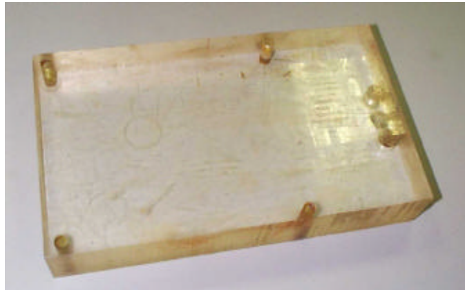
Figure 5.6 Plexiglas block used in the laboratory experiments. The dimensions of the Plexiglas block were 30.05 \times 18.05 \times 4.88 (cm) ( length \times width \times height ), of the same order as those of the Phenolite block.
