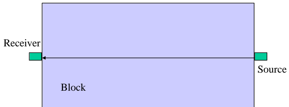
Figure 5.9 The laboratory setting for the measurement of horizontal velocity. The source and receiver transducers were fixed on the opposite sides of the Phenolite block to record direct horizontal travel time.
