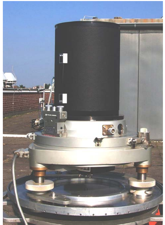
Figure 2.2: Digital zenith camera
