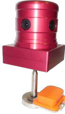
Figure 3.8: Assembly of Ladybug 2 omnidirectional camera (red with black lenses) and MTi inertial sensor (orange).
