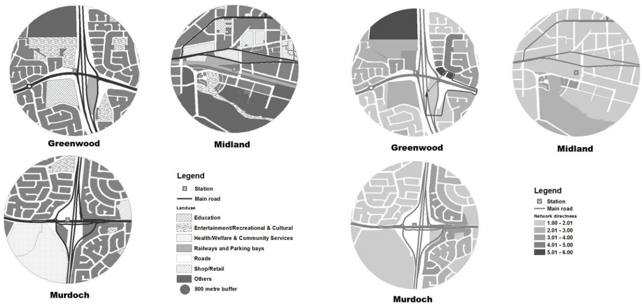
Figure 4: The Mixed Land-Use within 800m of Train Stations (left); Route Directness of a Train Station (right)
