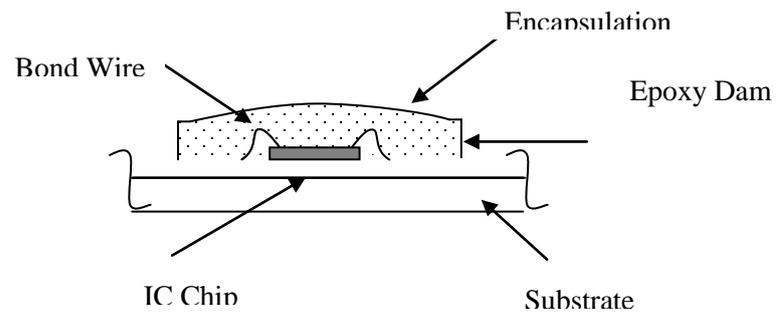
Figure 1 Encapsulation of COB packages
