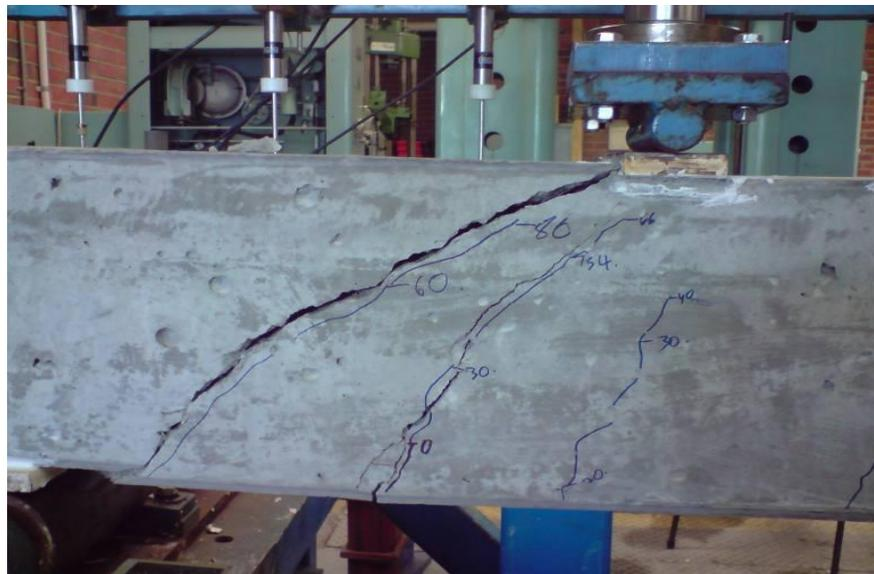
**Figure 8.** Crack formation at failure under shear test.
