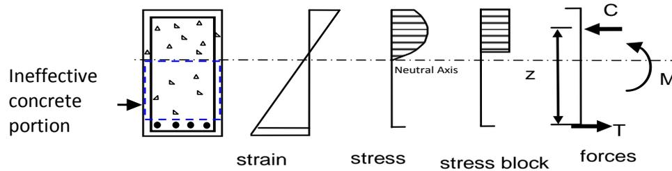
Figure 1. Strain, stress and force diagrams of a reinforced concrete section.
