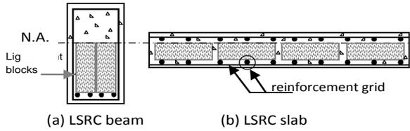
**Figure 2.** Reinforced concrete section with lightweight blocks infill.
