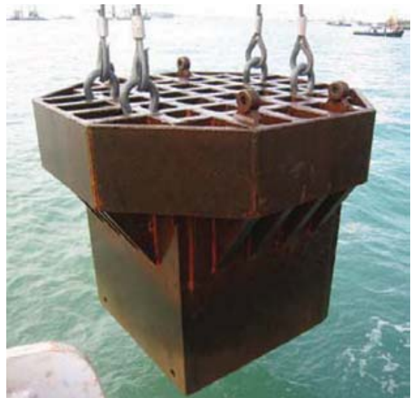
Fig. 4: Specially designed and fabricated offshore DR pounder (Chu et al., 2009)
