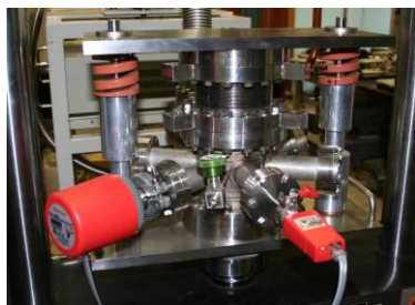
Fig 11 – Set up of the chamber supported by two steel columns with springs.
